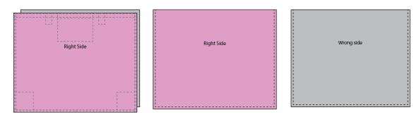
Turn Bag Right Side Out & mark corner pattern markings. Cut through all layers as shown below. Bring sides of box corners together and sew at ½ cm on Right Side of fabric, trim bulk and corners. Turn Bag Wrong side out and repeat ½ cm seams on Wrong Side.
