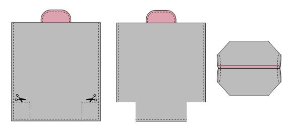
At the top edge of bag fold a 1 cm seam allowance to the wrong side, iron flat. Insert the straps at pattern markings under the folded seam. Pin in place, make sure pocket flap is flapped down before next step. Now fold top edge again 1 ½ cm towards the wrong side. Topstitch on wrong side close to edge as below. Now fold back handles and topstitch top edge, sewing handles down.
