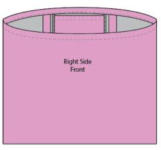
Fold Handles up & pin in place. Fold the Pocket Flap up and pin in place. Do a Final row of Topstitch close to the op edge, sewing handles and pocket flap into upwards position as shown below.
