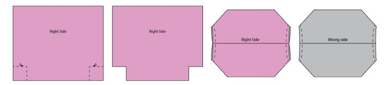
Turn Bag Right Side Out. Fold a  $\frac{1}{2}$  cm seam allowance to the Wrong Side all around top edge. Now Insert straps on wrong side under  $\frac{1}{2}$  cm folded seam. Insert Pocket in the same way as on pattern markings. Pin all in place.
